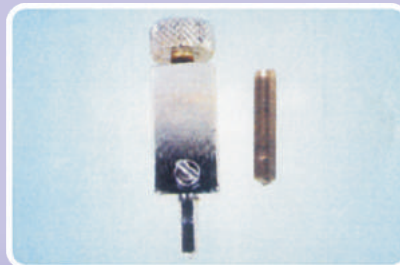
Round Cutter Pin Holder with spare pin.
