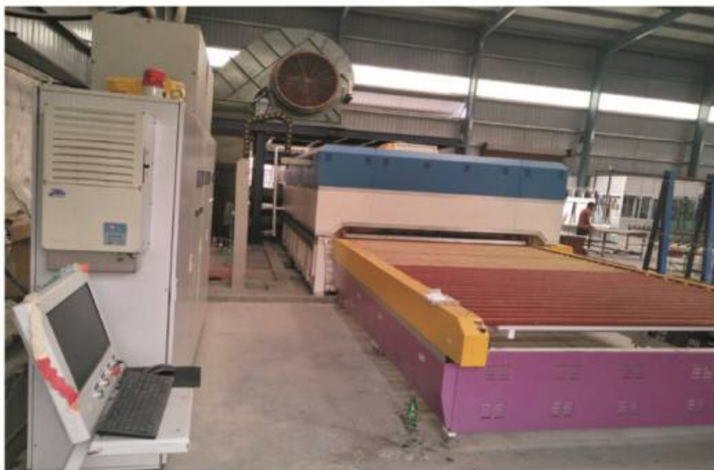
A Picture of imported horizontal tempering line set up by the company
